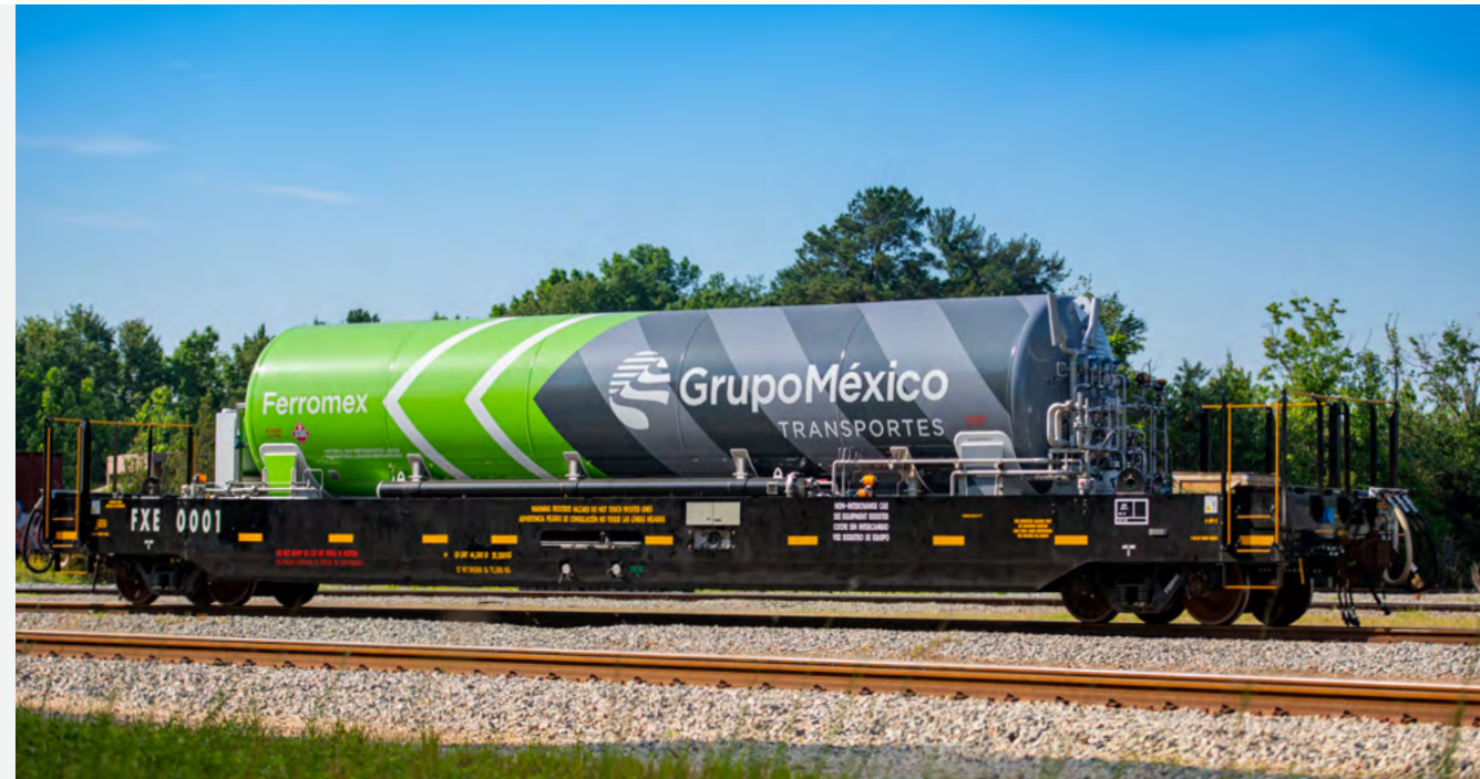
Tender with Liquefied Natural Gas for hybrid locomotives, Ferromex, Mexico.
